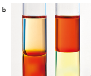
FIGURE 14.1.5 (a) When an alkene is added to aqueous bromine, the alkene reacts with the coloured bromine and the solution loses colour. (b) When an alkane is added to aqueous bromine, no addition reaction occurs and so the colour remains.
