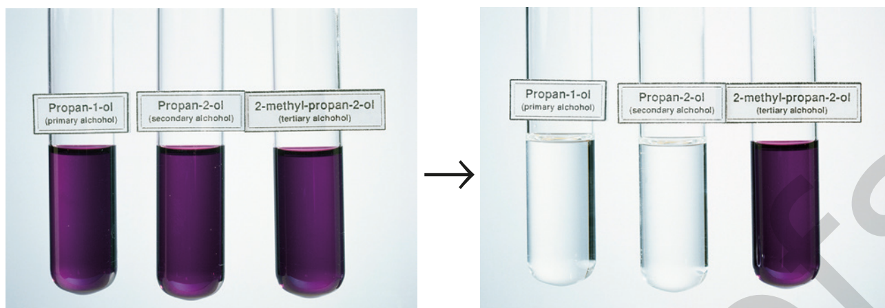
FIGURE 14.2.9 The strong oxidising agent potassium permanganate is deep purple in colour. On reaction with primary and secondary alcohols, the colour changes from purple to colourless. The tertiary alcohol is resistant to oxidation under these conditions and does not react, so the solution does not change colour.
